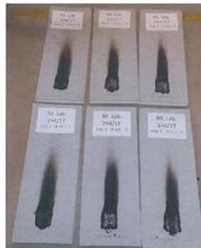
Picture 3: membrane surface after the test
